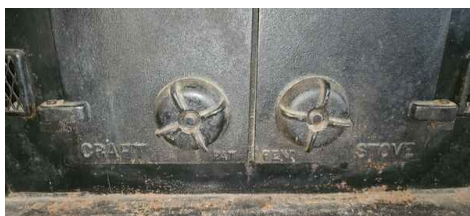
Air intake vents increase or decrease airflow into the firebox to adjust for woodburning intensity and duration.
