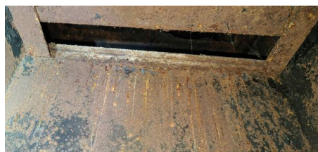
Steel elevated wood holder, allows wood to combust properly and burn completely.
